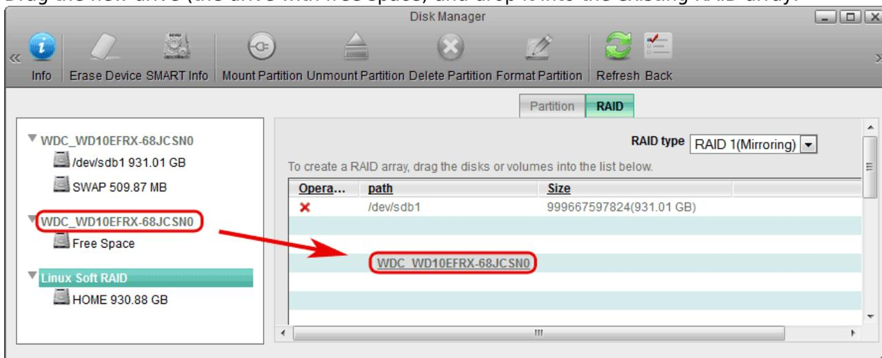
4. Scroll down and click **Rebuild**. This will create a partition identical in size to the existing drive already in the RAID array and start mirroring the data.
