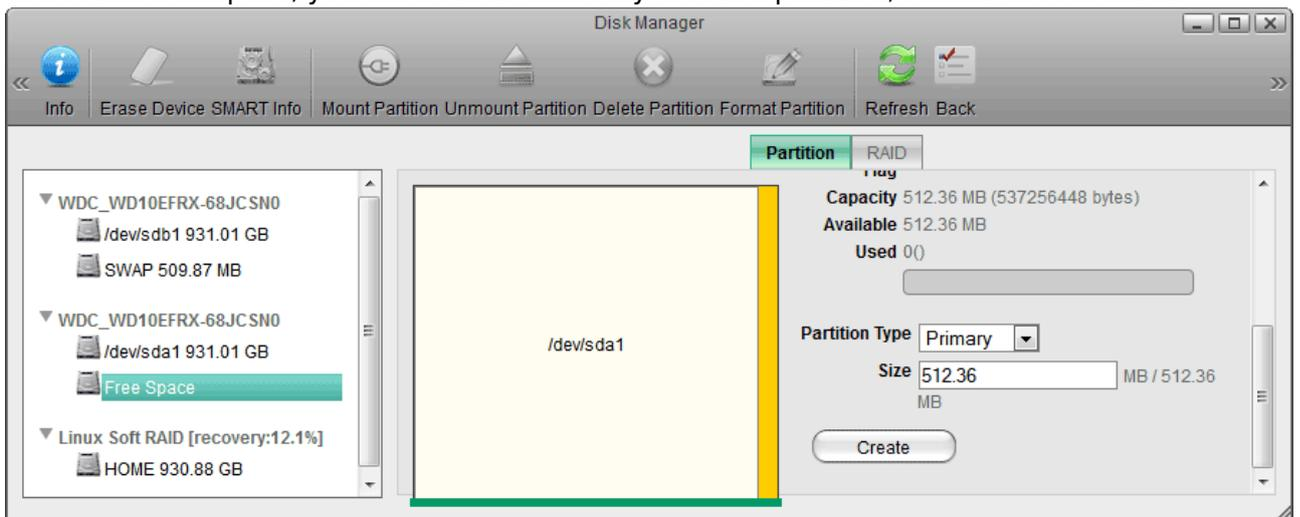
7. Assuming that the capacity of your new drive is identical to the existing drive, we suggest creating a SWAP partition. To do so, select the **Free Space**, open the **Partition** tab and click **Create**. The partition type and size can be left at default.
