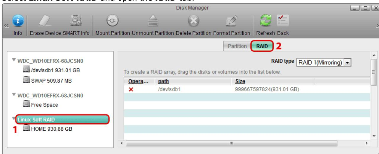
3. Drag the new drive (the drive with free space) and drop it into the existing RAID array.
