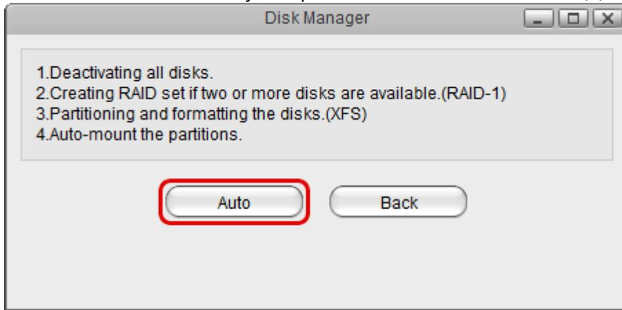
2. The installation wizard will deactivate all disks and if two drives are installed, it will create RAID 1 array. It will create a SWAP partition for the system, a partition for your data, format the drive(s) using the XFS file system and then mount the partitions.
