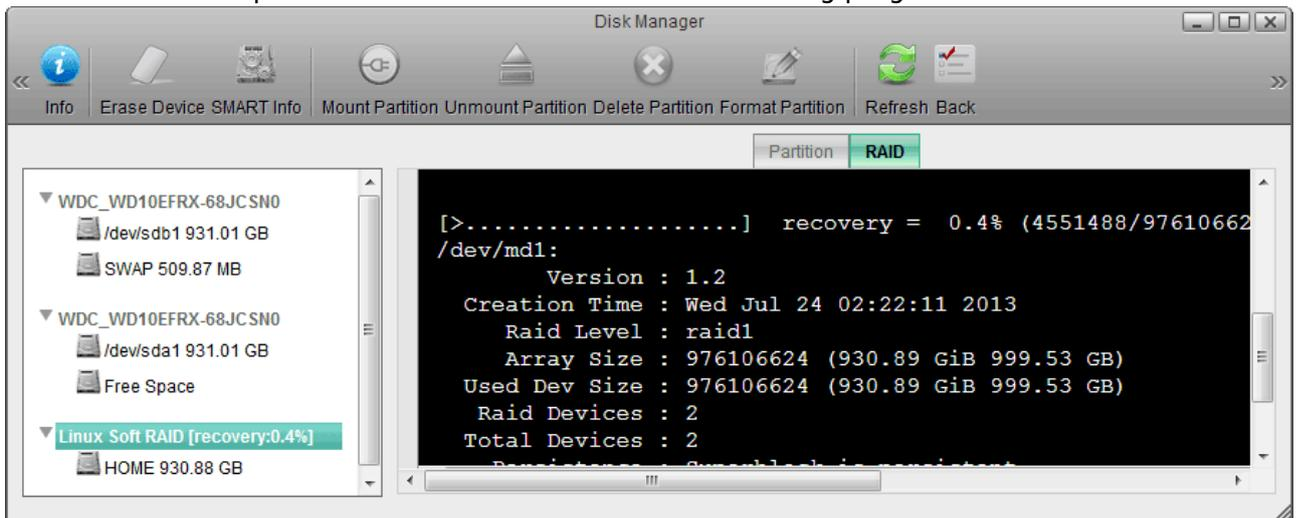
6. Depending on the capacity of the new drive, you will have some additional free space. If the capacity is identical to the existing drive, the remaining space can be used for SWAP. If the capacity is larger, you can create an additional partition for extra storage. Either way, to make use of this free space, you will have to manually create a partition, format and mount it.
