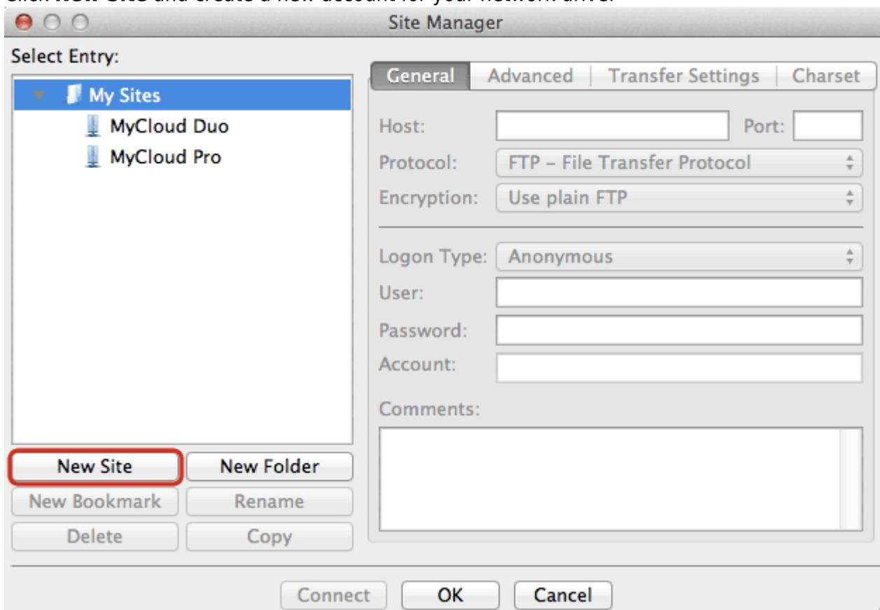
4. For the host, enter the **IP address** of your network drive (e.g. 192.168.33.30). Use the local IP address as seen under [Preferences > Server Info](#) but without the port number.
