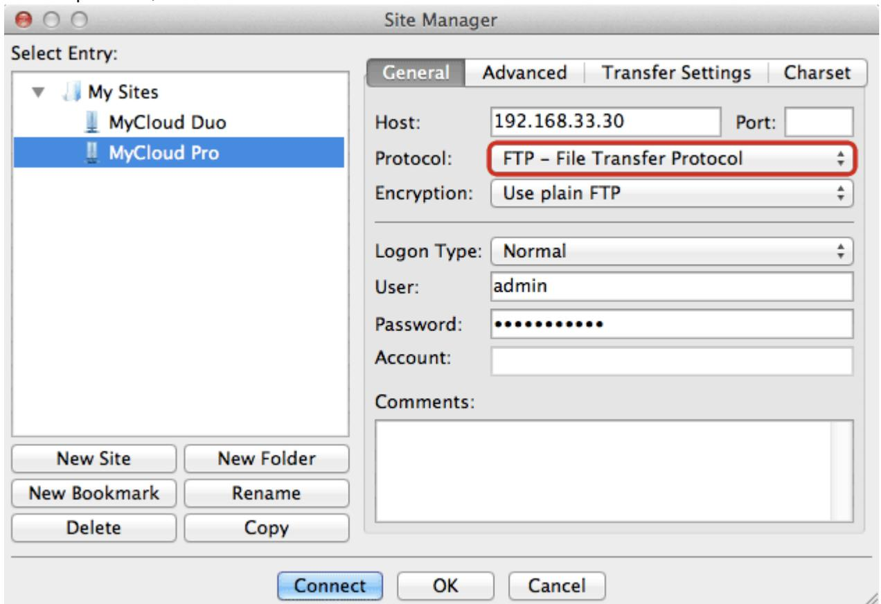
6. For the encryption, select **Use plain FTP**. If the FTP server is set to use SSL encryption, select **Require explicit FTP over TLS** instead.
