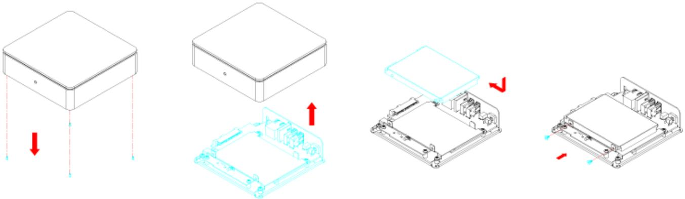
Replace the top enclosure. Fasten the screws on the bottom of the case, place the rubber feet over the screws and stick them on the casing to cover the screws.
