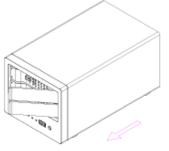
Install the hard drive, making sure the connector is facing the open side of the bracket. Slide the tray back into the enclosure and push the handle lightly into place.
