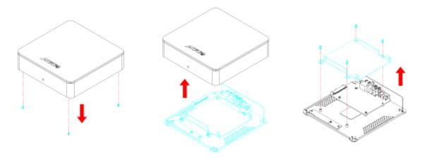
Install the hard drive in the HDD chassis and fasten the screws on the sides to hold it in place. Mount the HDD chassis and replace the top enclosure. Fasten the screws at the bottom of the case, place the rubber feet over the screws and stick them on the casing to cover the screws.
