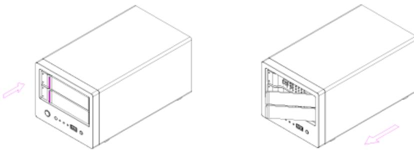
Install the hard drive, making sure the connector is facing the open side of the bracket. Slide the tray back into the enclosure and push the handle lightly into place.
